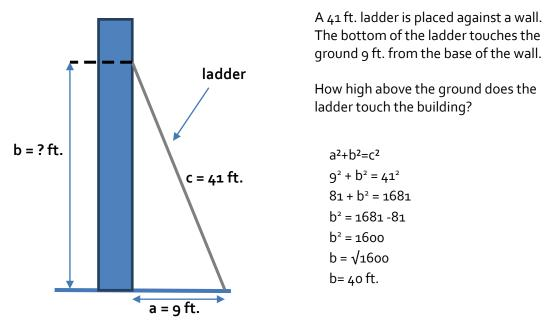
The standard rule of safety when positioning a ladder is that for every 4 units of height, to the point where the ladder leans against the wall, the base of the ladder should be 1 unit away from the surface on which the top rests. This ladder is not properly positioned to be considered safe. It touches the wall at 40 ft. The base should be 10 ft. from the wall and it is only 9.
