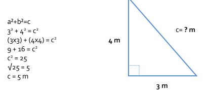
Here is an example of the theorem used in the case of ladder placement.
