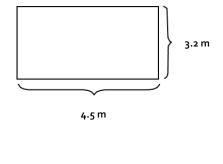
$A = L \times W$   $A = 4.5 \text{ m} \times 3.2 \text{ m}$  $A = 14.4 \text{ m}^2$
